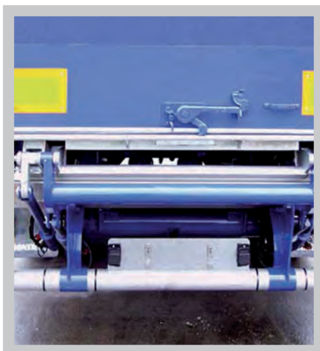
REP/4: 2 lifting + 2 tilting cylinders and automatic tilt
